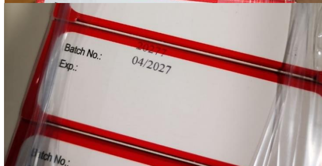
Carton with misaligned batch no. and expiry date
